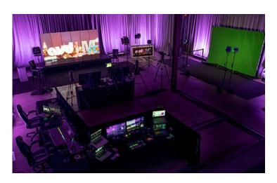
"I started playing with it and programming with it and realized that we could use the Aquilon for master control in the streaming studios. It was the perfect solution! The Aquilon RS1 is essentially a 12 M/E switcher, with a level of control and operability you don't find in broadcast switchers. It can handle multiple layers and complex content, and many people working remotely can log onto it at the same time."
