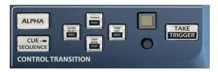
Into the control transition section, you can choose either to control the transition (default section behavior) or to control the cue sequence playback.
