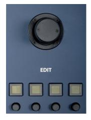
For all numerical settings, you can choose to update them roughly via the Joystick, finely via the encoders, or directly via the numpad. To enter a specific value via the numpad, press the button above the encoder to activate the numpad on the **EDITpad** and then enter the desired value. When ready, press the **ENTER** button to apply the new value.
