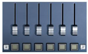
Below each fader you will find a scene button, you can use the left/right arrow to move this scene list. Each fader will transition the scene which is written on the button.
