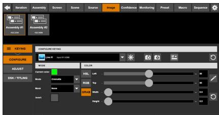
Keying setup can be done either by setting directly color references and tolerances or by using an assistant (**GRAB** button). When using the assistant, select the color area you want to mask and press the **PICK** button. Color areas are cumulative; if the results are not satisfactory, press the **RESET** button then grab another area.
