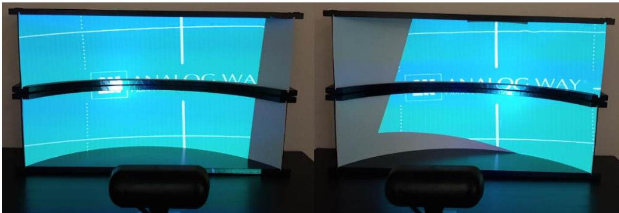
Fig. 77 - Autocalibration: test images after the initial calibration process (2 projectors)
