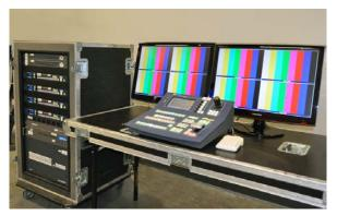
**Pulse** is a Multi-Layer Mixer Scaler Seamless Switcher with full digital in/out processing plus universal analog inputs. It offers 10 direct inputs including 2 fitted with DVI and 2 fitted with 3G-SDI. **Orchestra** is a powerful, intuitive and ergonomic Remote Controller designed to manage independently or simultaneously a variety of **Analog Way**'s Switchers as well as a variety of up-stream matrix devices.
